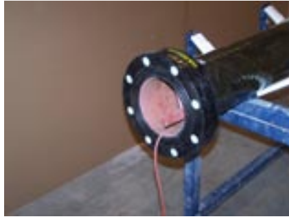
Photo 11 - Cure adhesive joint
