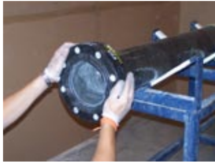
Photo 13 - Push flange onto spigot
